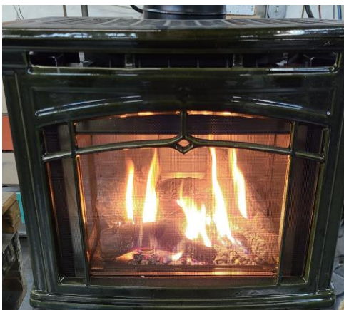
Figure 35 - Typical Burner Flame Appearance
