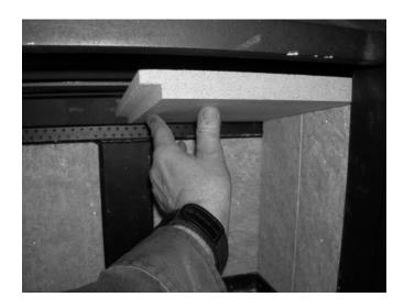
5) While lifting the rear portion of the right baffle, insert the left baffle by engaging the rear and tipping up the front. IMPORTANT – do not force the pieces as they could break or crack – they will fit together without forcing them into place. The two baffles will overlap at the center joint and sit in the grooves of the left and right stones.
