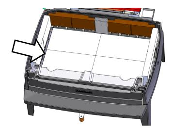
8) Install the three catalysts into the correct spot shown in the section view below. Orient the openings of the catalyst facing up, towards the top of the stove. The catalyst can go through the flue collar, or through the rear exit cover plate, depending on which configuration you are installing.
