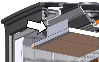
7) Place the bottom refractory stones into the stove.
