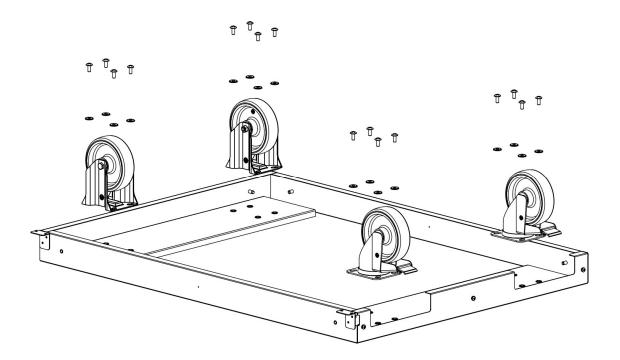
2- Put the shelf with wheels back in the original position. We recommend blocking the two wheels by activating the brakes. Take the left side of the cart and screw it with five M5x16 screws as shown in the image below. You may need the help of another person to hold the cart side.
