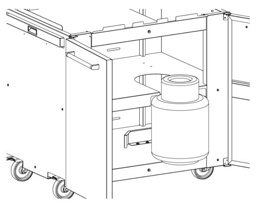
12- Stop the cylinder with the front support bracket. Fix it using two M5x16 screws and the respective 5x15 washers. The support bracket has two slots that allow it to slide until the bracket fits perfectly with the cylinder.
