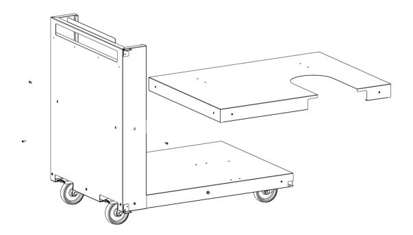
**4-** While keeping the intermediate shelf, place the right side and fix it to the intermediate shelf and to the bottom shelf using eight M5x16 screws.
