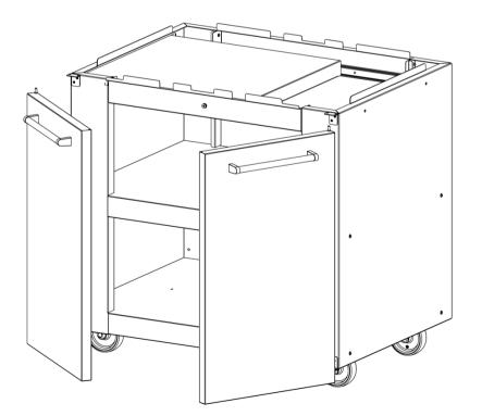
**9**- Mount the rear panel of the cart using five M5x16 screws as shown in the image below.
