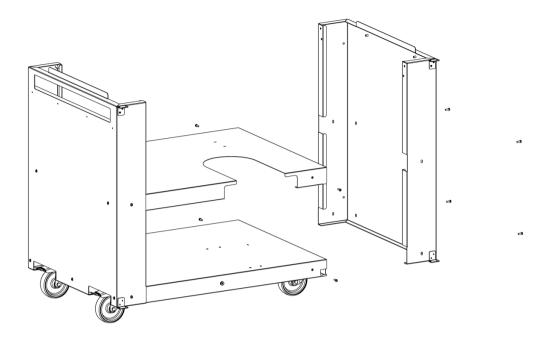
5- Take the two crossbars of the trolley with the guides already pre-assembled. Be sure the guides are properly closed. Place them between the two sides, taking care to position the one with the door closing magnets at the front. Fix them with four M5x16 screws per crossbar.
