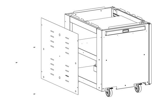
**10-** If you want to place the cylinder inside the cart, fix the back cylinder support bracket with two M5x16 screws and two 5x15 washers
