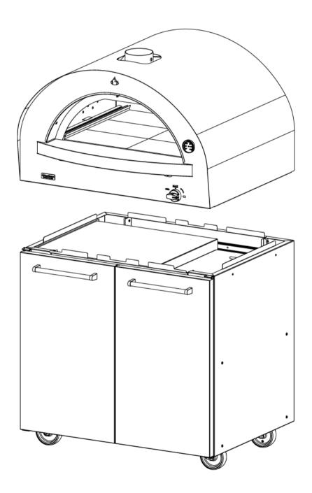
14- When the oven is safely placed on the cart, take the diaphragm and place it over the flue opening.
