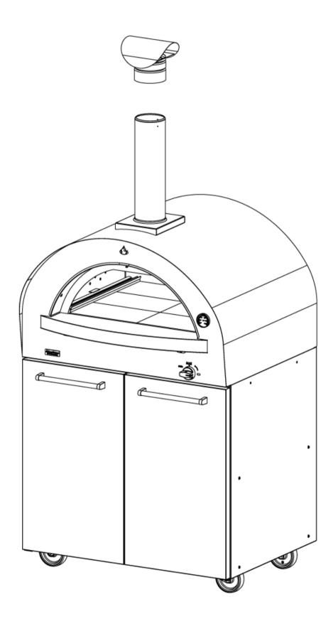
**17-** You can fix the cap to the flue using the 4.2x16 self-drilling screw supplied.
