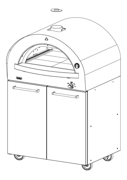
**15-** Take the chimney flue and insert it on the flue opening of the oven.
