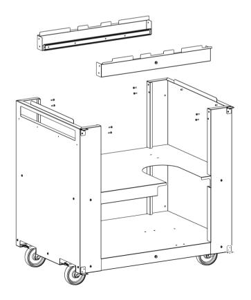
6- Pull out the guides and let them come out of the rectangular slot on the left side. Once outside you can assemble the side shelf, paying attention to the symbols. For the 80x60 oven, secure it with four M4x10 screws to the inserts showing the square symbol. For the 60x60 model secure the shelf with 6 M4x10 screws to the symbols showing a triangle. The 100x80 model will have its own side shelf to be fixed with four M4x10 screws.
