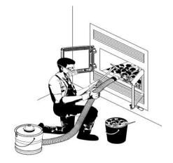
The chimney should be checked regularly for creosote build-up. Inspection and cleaning of the chimney can be facilitated by removing the baffle.
