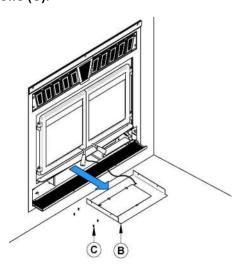
2. With a short square head screwdriver, remove the 4 screws (C) holding in place the heat shield (B).
