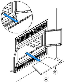
1. Remove the inner ash retainer and the floor 2. Using a power screwdriver and hex tip 5/16", remove the slab holder (D) and the left refractory slab (C).
