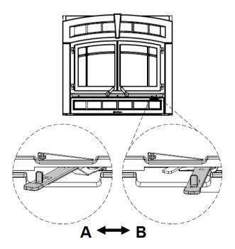
**Position A:** In this position, air supply is fully open. You should be using this position for :
