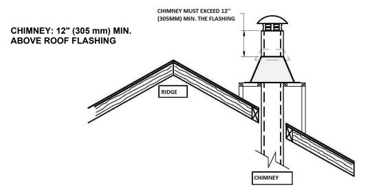
Note: The chimney chase on the roof must be the same size as the flashing.
