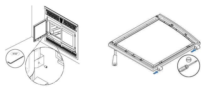
Using a flat screwdriver, turn the adjustable hinge rods in the direction shown to adjust the doors. Tighten all door hinge pressure screws when they are at the desired positions.
