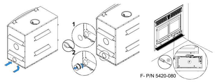
3. Flip the fireplace lower decorative louver. Install the blocking plate **(F)** included with the fireplace, on the front opening of the air control housing. Using a screwdriver, secure with four screws located in the user's manual.
