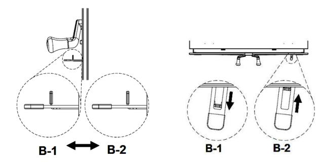
In the B position, it is also possible to close the air supply manually if a power failure occurs by pushing the small lever to the left.
