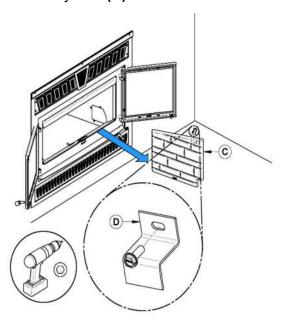
3. Remove the 4 bolts (E) holding the access door 4. Remove the thermodisc (G) by unscrewing the (F) with a 1/4" ratchet.
