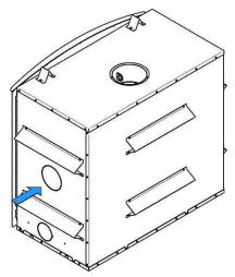
This kit allows distributing heat to another room up to 50 feet (15 m) of the fireplace. The insulated flexible pipe (not included in the kit) must be HVAC type pipe and must comply with ULC S110 and/or UL 181, Class 0 or Class 1 Standards and must withstand temperatures up to 250°F.
