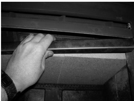
Figure 19a – Removing / Replacing the Baffle
