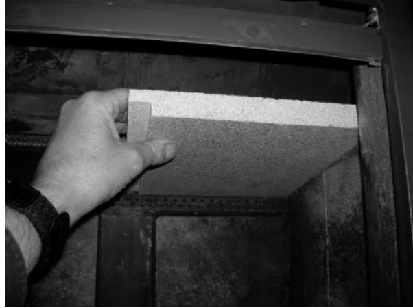
Figure 19b – Removing / Replacing the Baffle
