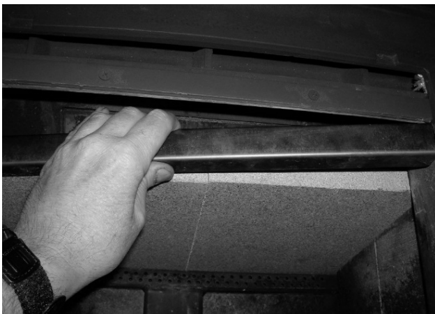
Figure 16 - Removing/Replacing the Baffle for Inspection
