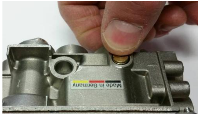
Figure 23 – NG Low Flow Screw Removal
