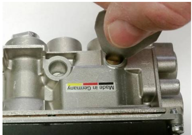
Figure 25 – Tighten LP Low Flow Orifice
