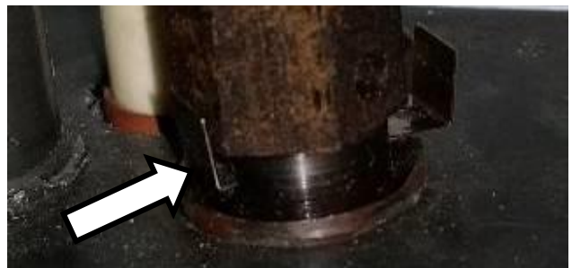
Figure 27 – Loosen Tower and Slide Pilot Gate to Rear of Pilot Tower (LP position)
