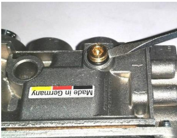
Figure 22 – Low Flow Orifice Removal – O-ring
