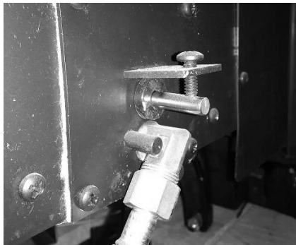
Figure 13 – Air Shutter Adjustment
