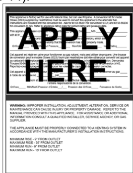
Figure 14 – Rating Plate Conversion Label Location
