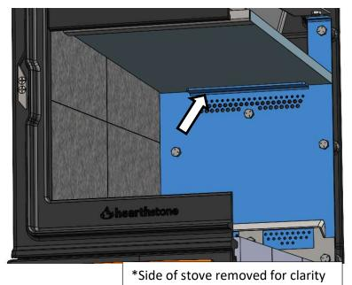
5. Align the front edge of the baffle into the baffle retainer. Push the baffle retainer to the rear of the stove and down into its retaining slot. Look down through the cook plate hole to easier see the movement of the baffle retainer.
