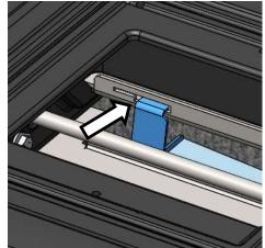
6. Reinstall the cook plate after the baffle is replaced. Go through the break in fire procedure as defined in the manual for the initial fire to properly cure the baffle.
