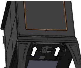
2. Install the rear heat shield by hooking the top edge of the heat shield under the top rim of cast iron. Line up the two holes in the bottom flange of the heat shield and reinstall the two previously removed screws to secure the shield in place.
