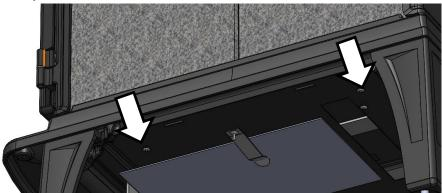
2. Hook the top edge of the heathsield under the rim of the cast iron top. Align the bottom flanges of the heatshield into the slots in the bottom sheild from step 1.
