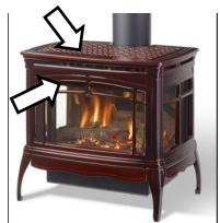
2) Locate the front glass retention clips along the top edge of the front glass. Using two 7/16" wrenches, remove the nut from the spring retention bolt. Be careful when removing the nut, the spring is under tension!
