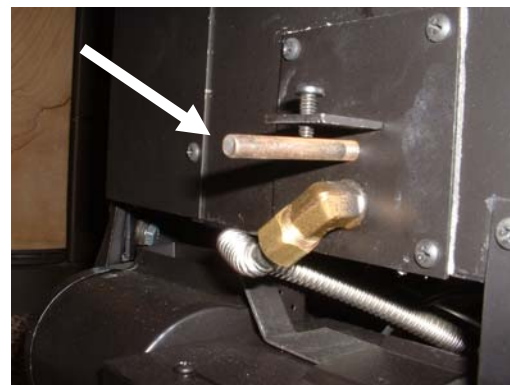
Photo 36 – Air Shutter Closed
