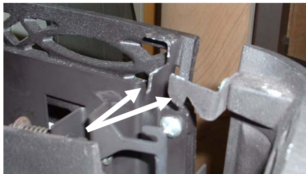
Photo 9 – Front Panel Mounting Tang Detail
