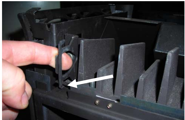
Photo 12 – Glass Spring Clip Detail
