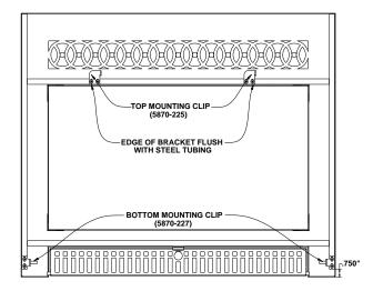
7. Attach the Vision Façade by lining up the two receiving bars located on the bottom of the Façade with the two hook shaped slots on the bottom of the DVI 32 Insert. Drop the bars into the slots and push the Façade toward the firebox until it "clicks" and locks into place (see illustration).
