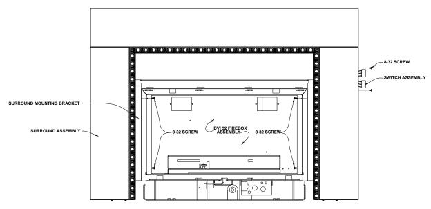
3. Align the screw holes in the side of the insert with the screw holes in the L-Shaped Brackets on the Surround assembly. Work on one side of the assembly at a time. Lift one side up slightly to line up the holes. There are four screw holes on each side, two large and two small. The 8-32 screws will need to be inserted into the smaller holes, leaving the larger holes open for the optional accessory screen. Repeat on the opposite side.
