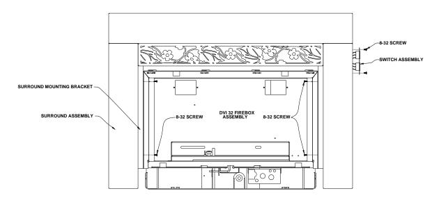
3. Align the screw holes in the side of the insert with the screw holes in the L-Shaped Brackets on the Surround assembly. Work on one side of the assembly at a time. Lift one side up slightly to line up the holes. There are four screw holes on each side, two large and two small. The 8-32 screws will need to be inserted into the smaller holes, leaving the larger holes open for the optional accessory screen. Repeat on the opposite side.
