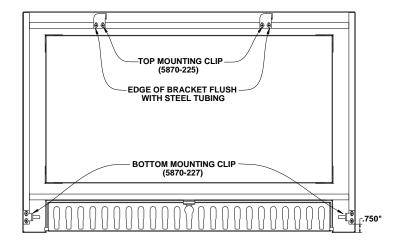
8. Attach the Silhouette Façade by lining up the two receiving bars located on the bottom of the Façade with the two hook shaped slots on the bottom of the DVI 32 Insert. Drop the bars into the slots and push the Façade toward the firebox until it "clicks" and locks into place (see illustration).
