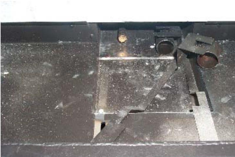
Photo 4 Left shutter moved to the side to allow access for orifice change. Repeat on right side.
