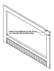
4. Attach the right extrusion. Align the (3) holes in the right extrusion with the (3) holes on the right side of the façade. Be sure the extrusion edges are fitting tightly against the façade and rivet the two pieces together. **NOTE**: It is recommended that the top extrusion be held in it's location while fastening the right extrusion to ensure correct alignment in the corners.
