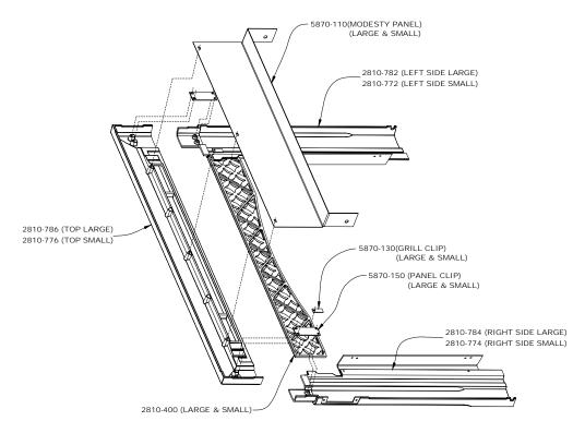
4. Use the two steel Grill Clips (steel clips with one hole each) to secure the Façade Grill to the Side Panels. Align the holes in the Grill Façade with the holes in the Grill Clips. The Grill Clips will overlap the Side Panels. While aligning the Façade Grill to a position level to the Side Panels, insert and tighten two 8-32 screws through the clips and into the Façade Grill. See illustration for details.
