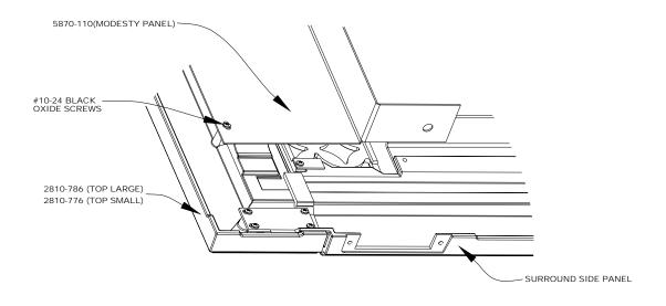
7. Before attaching the assembly, remove the glass from the insert. To remove the glass, pry up the four retaining clips. Lift the glass and frame up and off of the firebox. This will give you enough room to install the Surround assembly.
