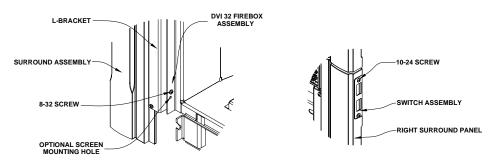
9. Align the screw holes in the side of the insert with the screw holes in the L-Shaped Brackets on the Surround assembly. Work on one side of the assembly at a time. Lift one side up slightly to line up the holes. There are four screw holes on each side, two large and two small. The 8-32 screws will need to be inserted into the smaller holes, leaving the larger holes open for the optional accessory screen. Repeat on the opposite side.
