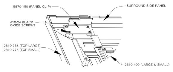
6. Lay the Modesty Panel onto the assembly with the flat side down. Line up the holes in the Modesty Panel with the preexisting holes in the Top Panel. Before attaching the Modesty Panel, make sure the flanges of the Modesty Panel are placed on the outside of the L-Shaped Brackets. Secure it with three 10-24 (black oxide) screws. Some Modesty Panels have five holes; it is only necessary to use three of the screws to mount the Modesty Panel.
