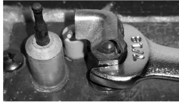
Figure 13 – Loosening Pilot Tower
