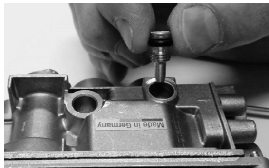
Figure 10 – NG Low Pressure Screw Insertion
