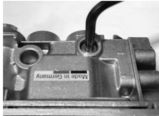
Figure 8 – Loosening Low Pressure Orifice
