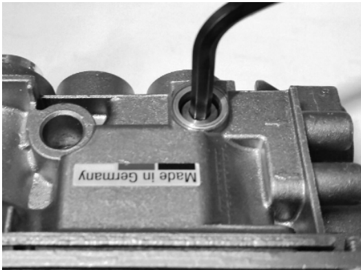
Figure 12 – Tighten NG Low Pressure Orifice
