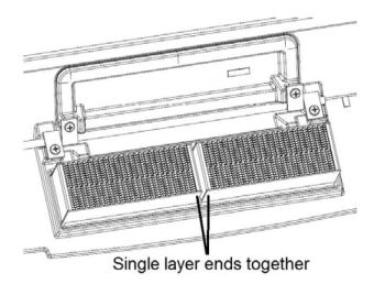
9. Heat the stove slowly during your next fire to allow the gasket and catalyst to break in together.
