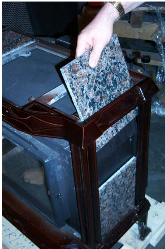
Figure 1- Inserting the Side Stones
