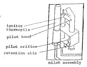
**WARNING:** Servicing of gas control, appliances, systems and leak testing must be PERFORMED BY QUALIFIED PERSONNEL ONLY.
