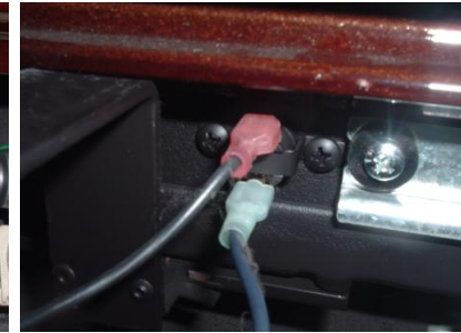
Photo #5: Wire from Rheostat to snap switch.
