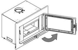
Hold the fire screen by the two handles and bring it close to the door opening.
