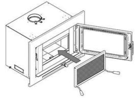
Lean the upper part of the fire screen against the top door opening making sure to insert the top fire screen brackets behind the primary air deflector.
