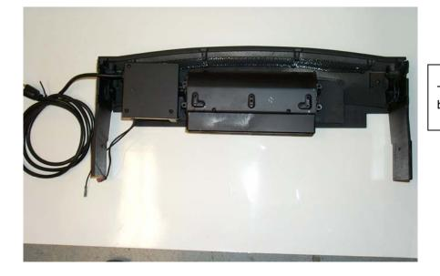
**Photo #4** The ash lip housing with the blower in place.
