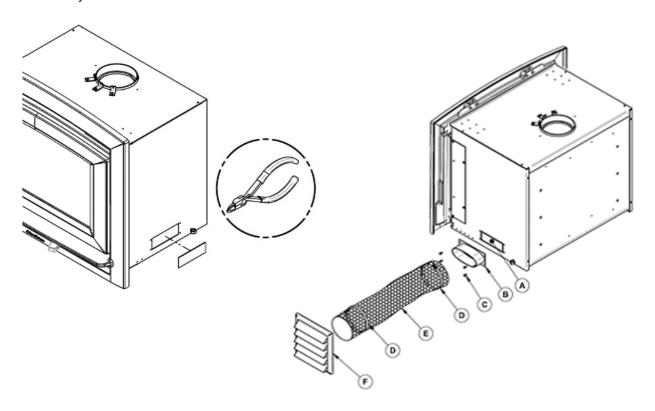
Then, install the fresh air kit adapter (B) using 4 screws (C). Secure the 5" flexible pipe 1 (E) to the adapter (B) using one of the adjustable pipe clamps (D). Secure the other end of the pipe to the outside wall termination (F) using the second adjustable pipe clamp (D). The outside wall termination (F) must be installed outside of the building.
