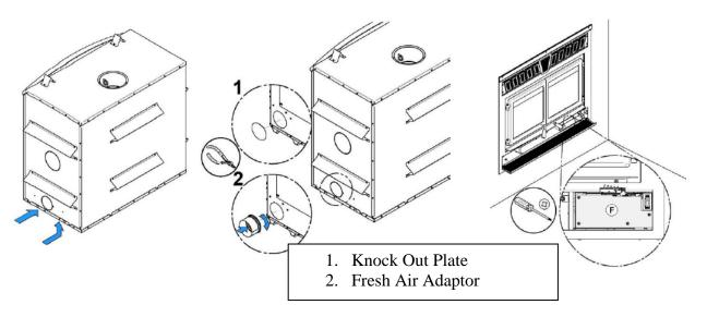
(2) Open the lower access door on the front of the fireplace and install the blocking (provided with the stove) over the original air intake opening. Secure the blocking plate by turning in the four screws with the phillips screwdriver (see illustration above for plate location).
