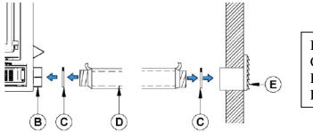
B: Outside Air AdaptorC: Hose ClampD: Insulated Flex LineE: Termination Cap
