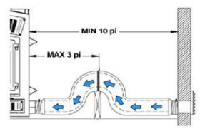
(4) Using the jig saw or hole saw, cut the opening in the outside wall to install the air intake cap. The hole will need to be just slightly larger than the 5 inch diameter of the connector pipe. Slide the termination cap through the hole in the wall as shown below. Secure the termination to the outside wall with screws.
