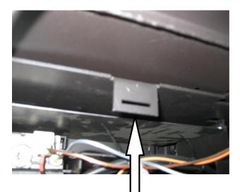
Photo #4 – Blower Tab Mounting Slot
