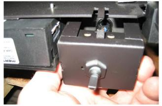
Photo #8 – Slide Rheostat Housing onto Tab
