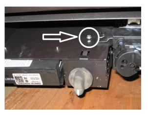
Photo #8- Tilt Valve Tray Down and Install Screw
