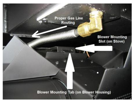
Photo #4 - Blower Tab Inserted in Mounting Slot
