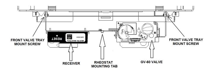
Figure #2 - Rheostat Mounting Tab
