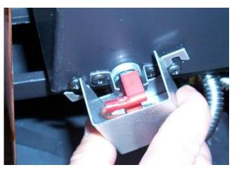
Photo #5 - Spade Terminal Connections
