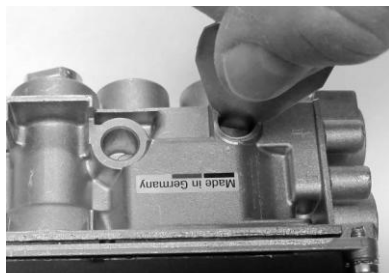
Figure 8 – Tighten LP Low Pressure Orifice
