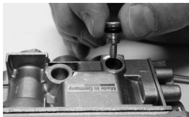
Figure 6 – NG Low Pressure Screw Removal
