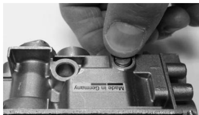
Figure 6 – NG Low Pressure Screw Removal
