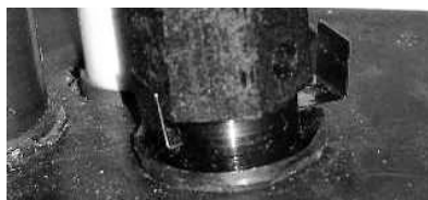
Figure 10 – Loosen Tower and Slide Pilot Gate to Rear of Pilot Tower (LP Position)
