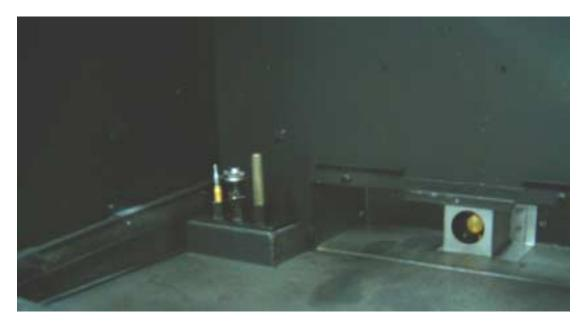
Photo shows Pilot assembly (left) and air shutter with burner orifice (right) in the firebox after the pan burner has been removed.
