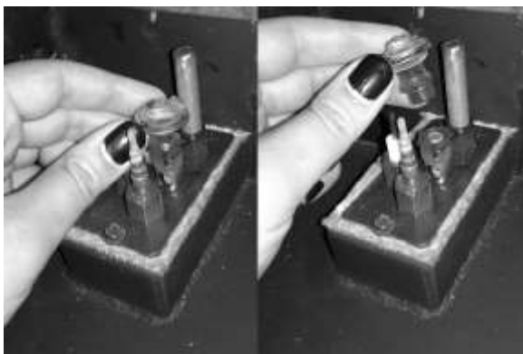
Figure 7 – Removing Pilot Burner Hood
