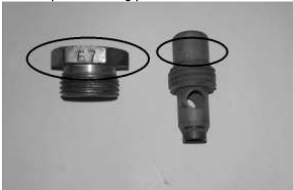
Figure 2 – Orifices, Marking Locations
