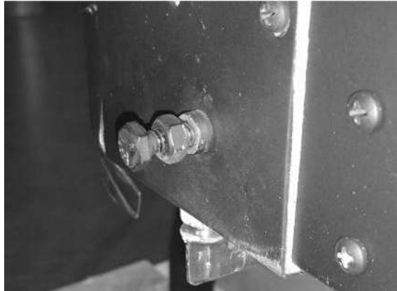
Figure 14 – Air Shutter Adjustment
