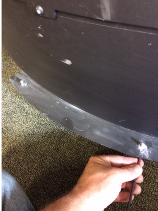
Figure 2 – Removing set screw/posts
