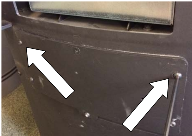
Figure 3 – Removing set screw/posts
