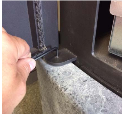
Figure 1 – Removing set screw
