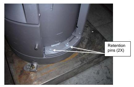
Figure 1: Bottom stone retention pins
