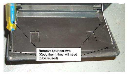
Figure 5. Front Lower Panel Installation
