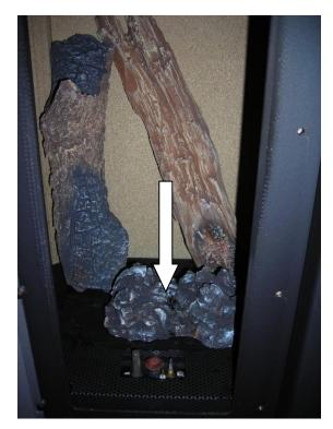
3. Locate and install the ember pile. This piece has two holes underneath that fit over two posts in the center of the burner top.
