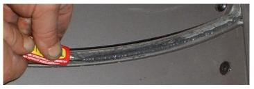
Figure 3: Apply Gasket Adhesive
