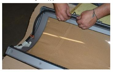
Figure 4: Install Gasket
