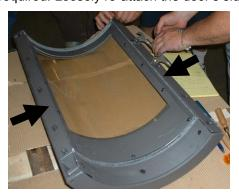
Figure 2: Loosely Attach Side Plates
