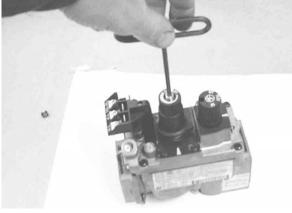
Photo #1 Remove the plug on the face of the Hi/Lo knob.
