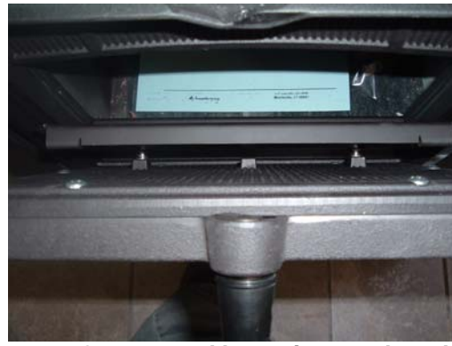
Figure 4: Gap created by springs and washers
