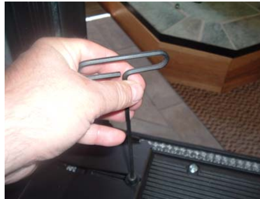
Figure 2: Bolt removal using allen wrench
