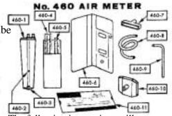
The Dwyer 460 Air Meter is capable of measuring draft and air velocity. The following instructions will only explain the procedures for measuring draft. For further information on measuring air velocity see the instruction card enclosed with the unit. *The only way to effectively separate the functionality of the stove from the functionality of the chimney is to measure draft in the chimney system.*
