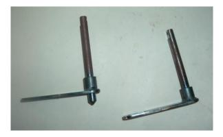
Photo # 1 Left: Original Primary Air Linkage Right: New Primary Air Linkage (provided in this kit)
