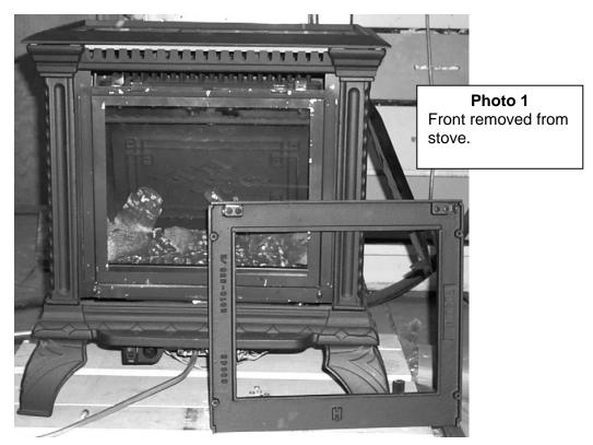
Figure 1 - Removal of Front
