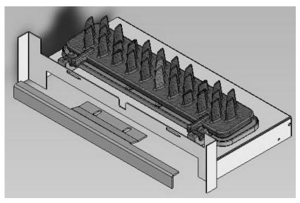
Figure 3 - Inserting the shield
