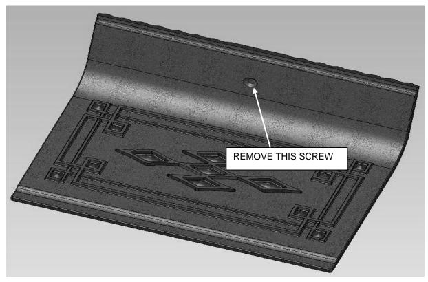
Figure 2 - Removing the baffle screw
