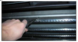
8) Move the baffle so that the indented lip will rest on the front baffle support when the baffle is properly placed. Adjust the cotter pins so that they drop through the holes in the secondary air tube. Bend the cotter pins so that the baffle will not move out of position.
