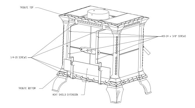
Tribute With Heat Shield Brackets and Shield Extension Plate Installed
