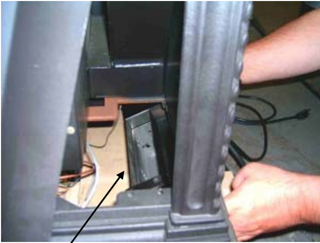
Photo #3 Rotate the blower so that the open end is facing up.
