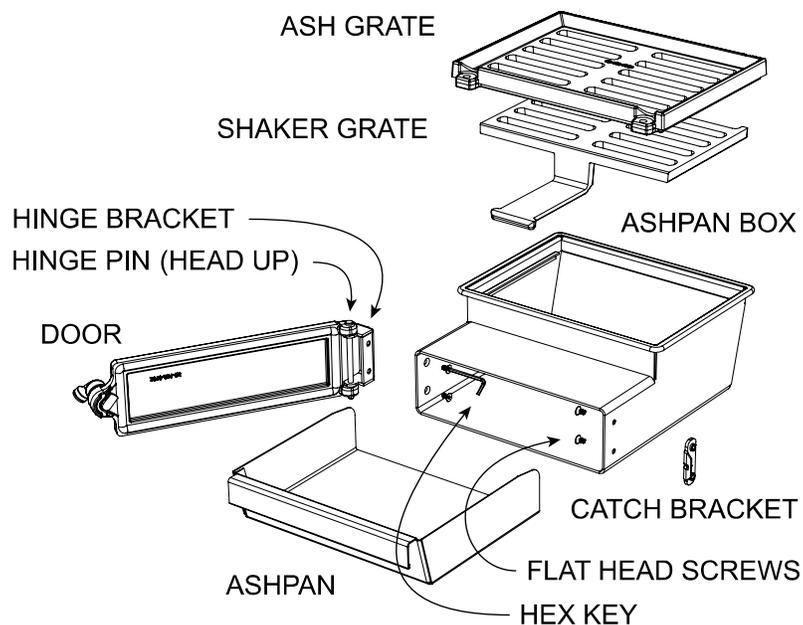
4. Remove the plastic keepers from the top flange of the ashpan box. These plastic sleeves hold the gasket in place during shipping. **DO NOT INSTALL THE ASHPAN BOX WITHOUT REMOVING THE KEEPERS.**
