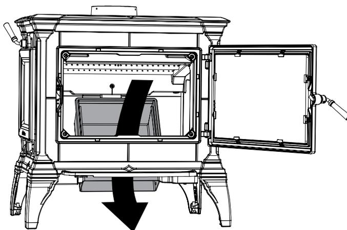
6. Install the shaker grate and ash grate:
