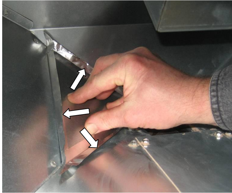
Figure 7 – Press Slider down with one hand and press tape down to hopper bottom at each side center with the other hand (see arrows). Place finger on Slider surface and slide from Slider toward tape to lay tape flat onto hopper bottom.
