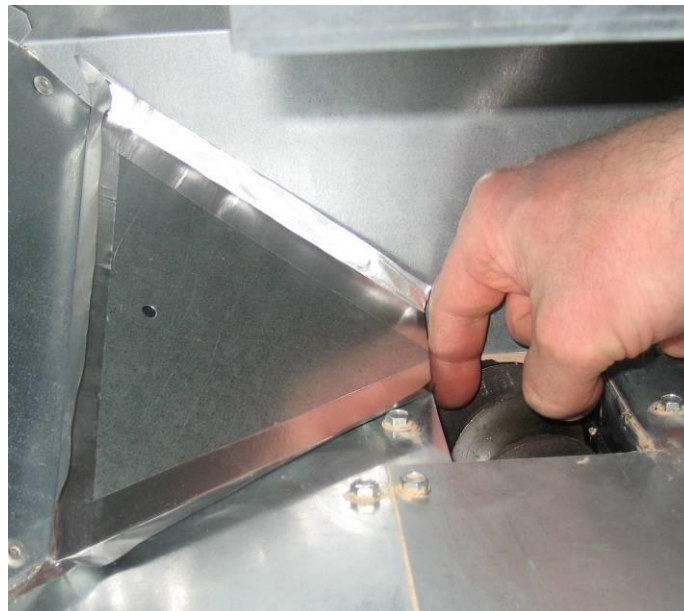
Figure 6 – Align Slider short side with Auger opening
