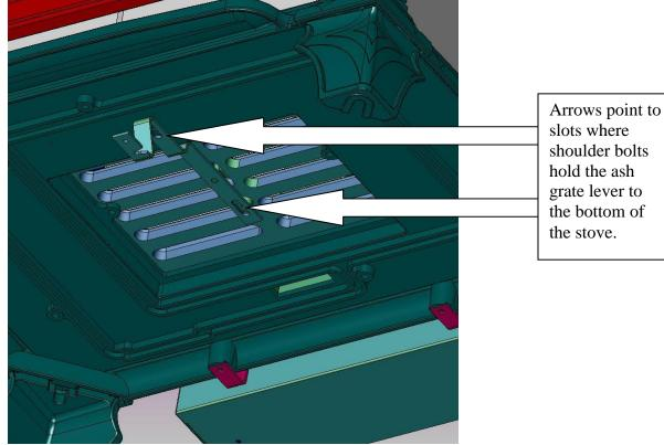
slots where shoulder bolts hold the ash grate lever to the bottom of
