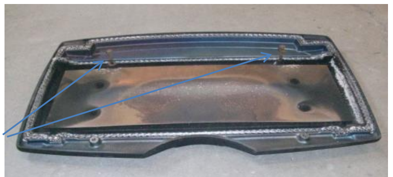
Front end of casting - showing 2 loosened nuts (View of top casting shown upside down)
